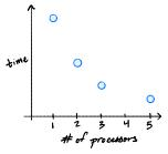
Find prediction rule  $H(p) = \frac{t_{NS}}{p} + t_{S}$  by minimizing MSE.
